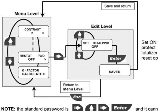
Set ON the Restot PWD to the resettable totalizer from undesired reset operations.
