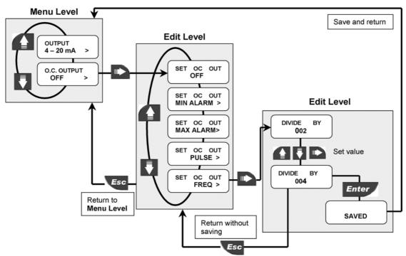
In FREQUENCY mode the O.C. output will simulate the sensor frequency divided by the set value. Enter any value between 002 and 255.
