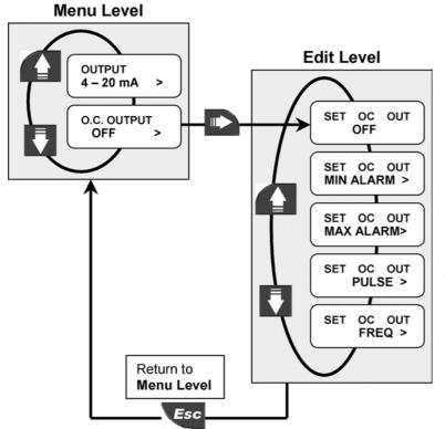
The mode of operation for the Open Collector Output (OPT) can be selected between different options: MIN alarm, MAX alarm, volumetric Pulse or Frequency.
