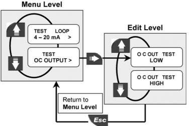
Manually toggle the status of the Open Collector (OPT) output for testing
