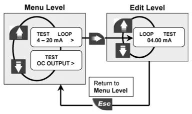
Manually simulate any output current value to test current loop
