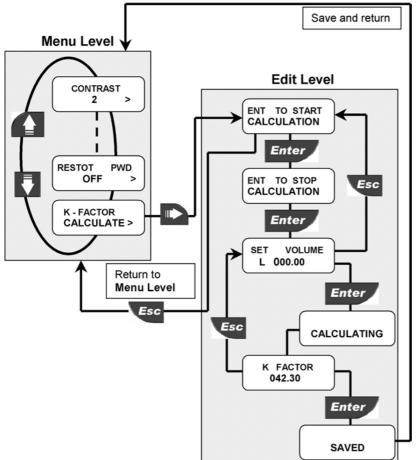
Press ENTER to start calculation. Switch on a pump or open a valve. F9.00 starts counting pulses from the sensor.
