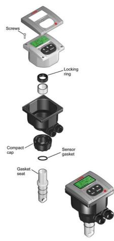
The compact mounting kit F9.KC1 includes the compact plastic adapter with gasket for IP65 watertight installation, the sensor gasket, the compact cap, the locking ring and four fixing screws.
