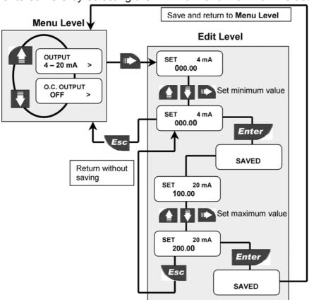
F9.00 will allow any value from 0.0000 to 99999 and the beginning of the measuring range can be larger than the end of it (inverted output signal).
